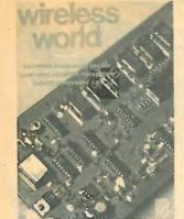
Front cover shows the 200MHz frequency meter which provides the main project for construction in this issue. See inside for Part 1.
